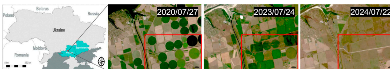
FIGURE 2 PlanetScope imagery of irrigation canal networks before and after the Kakhovka dam destruction on 6 June 2023, shows formerly dark, filled canals turn to dry canals in 2024 (46° 42' 42.41" N 33° 22' 20.85" E).
