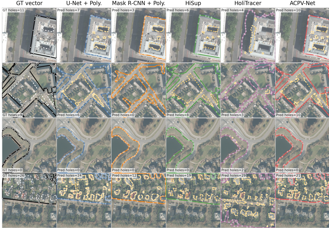
Figure 8: Additional qualitative vector predictions with segmentation and representation-to-vector baselines. Rows show the four object categories in the same order as Figure 7. Columns show the ground-truth vector, U-Net + Poly. and Mask R-CNN + Poly. (Seg.), HiSup, HoliTracer, and ACPV-Net (Rep.). Prediction columns contain no ground-truth overlay, so the figure directly shows each method’s predicted exterior ring, interior rings, and vertices.
