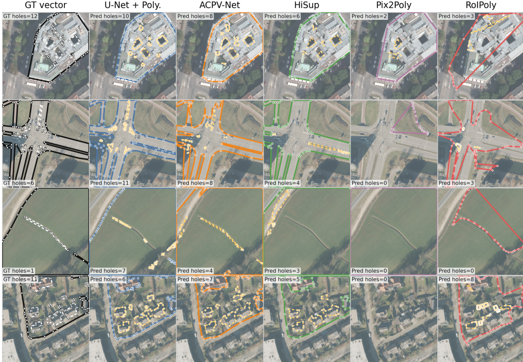
Figure 11: Additional qualitative vector predictions including direct vector decoders. Columns show the ground-truth vector, U-Net + Poly. ( Seg. ), ACPV-Net and HiSup ( Rep. ), Pix2Poly and RoIPoly ( Direct ). Direct decoders often produce simple or distorted exterior rings and miss many interior rings, while representation-to-vector methods recover more local structure but still fail to match the complete ring topology.
