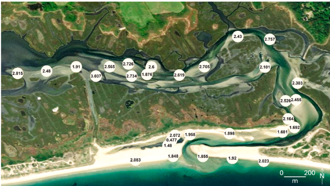
Fig. 12. Fining mean grain size ( \Phi ) trend suggests a new landward transport of sediment through the inlet and into the back barrier.
