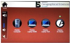
3. Now tap on the Display Air Media button. This will switch the projectors source to the streaming device.
